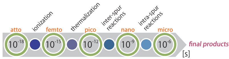
Fig. 1.7 | Time-scale of radiation-induced reactions.
