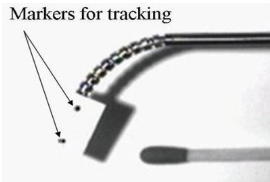
Fig. 2.22 Image processing for the evaluation of the positioning accuracy [57]
