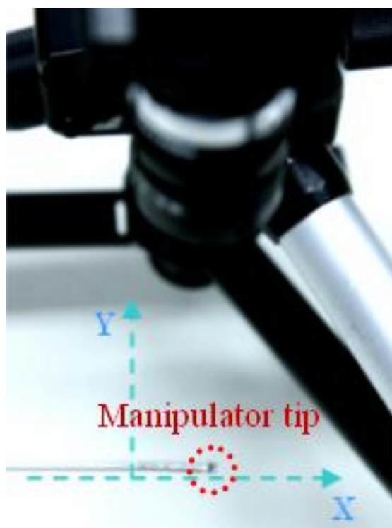
Fig. 3.2 The camera position and the coordinate system of one unit manipulator
