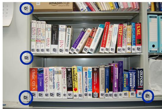
Figure 4.11: Visual tags with blue circles that indicated the corners of the bookshelf
