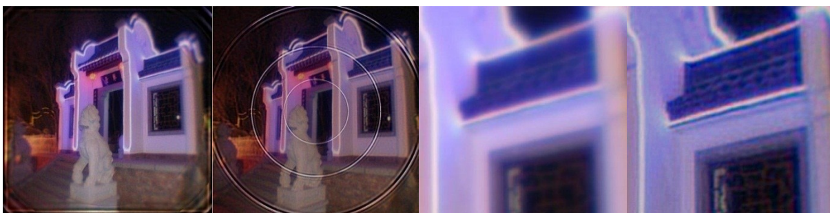
(e) Deblurred without larger black background (f) Deblurred without boundary expansion (g) Blurred area 1 enlarged (h) Deblurred area 1 enlarged
