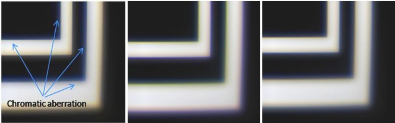
Image before LCA correction Corrected by first order Corrected by third order
