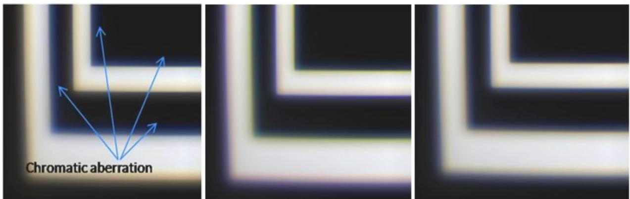
Image before LCA correction Corrected by first order Corrected by third order Fig.4.8 Image comparison before and after LCA correction for region 3
