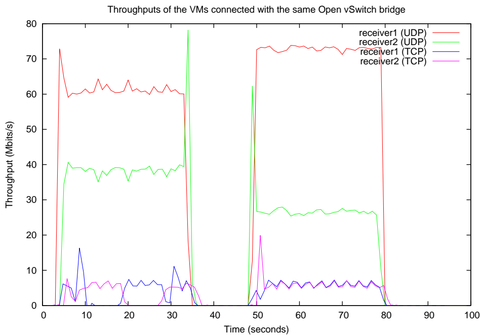
Figure 4.3: The traffic of the instances on the ratio-based rate limiting environment
