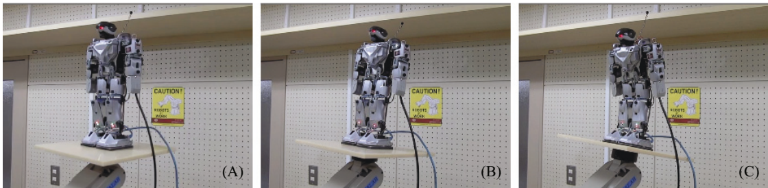
Figure 5-26. Actual robot motion when the robot arm makes the back slope (Humanoid robot: With balancing control)
