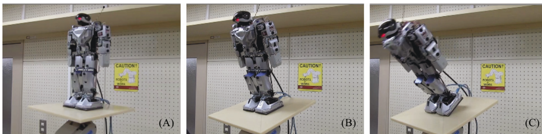
Figure 5-22. Actual robot motion when the robot arm makes the front slope (Humanoid robot: Without balancing control)
