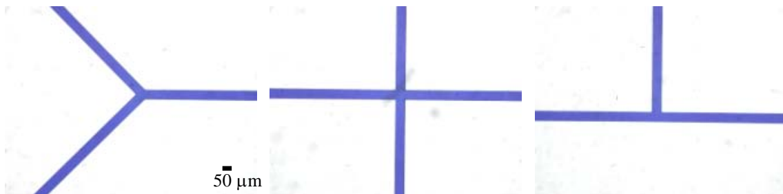
Fig. 4.16: Flow behavior at the Y-junction, the cross-junction and the T-junction in the fabricated microchip using methylene blue aqueous solution [5].
