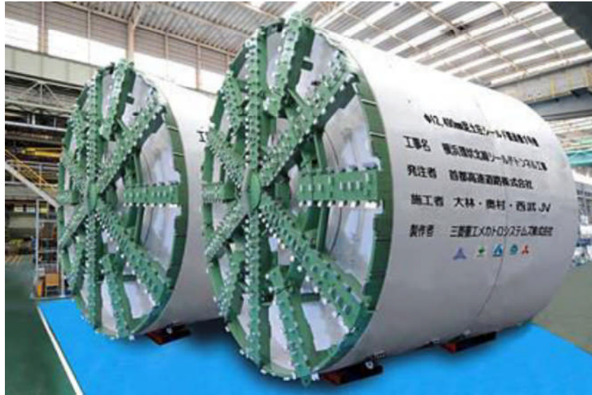
Figure 4.5. Used EPB shield machines for tunneling of Yokohama Circular Northern Route (reproduced from the http://radiate.jp/20111111/kouza34/# )
