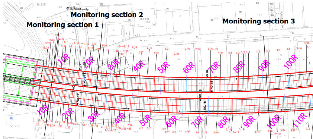
Figure 4.12. Date of excavation, ring numbers (shown by R), and monitoring sections.
