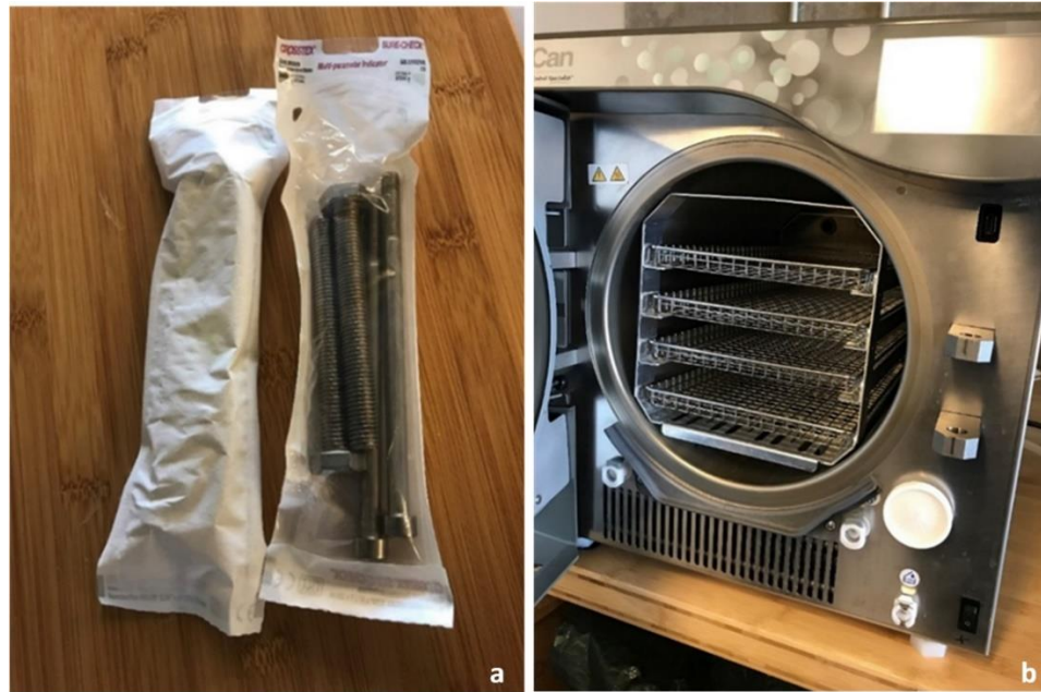
Figure 3.1 a) The transparent plastic side and the steam permeable paper side of the packed pouches. b) The trays inside the chamber without any load inside
