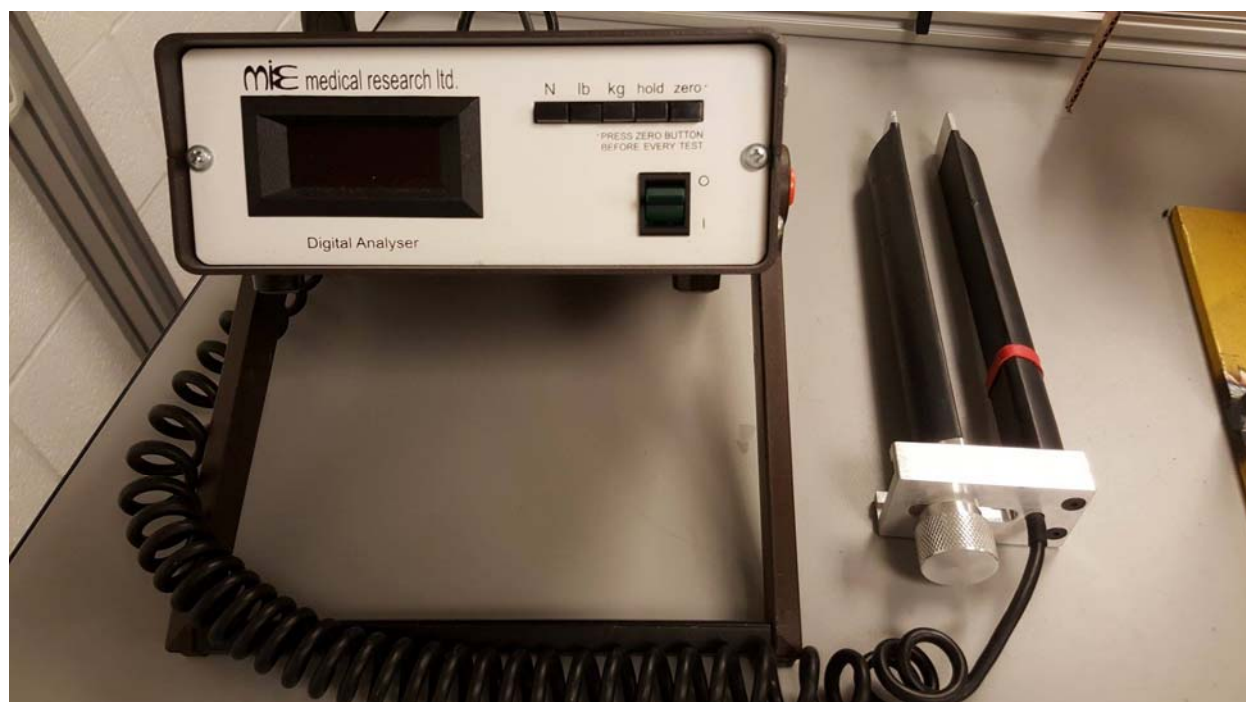
Figure 10: Hand-grip dynamometer (MIE Medical Research Ltd., Leeds, UK) used to measure grip strength in Newtons.
