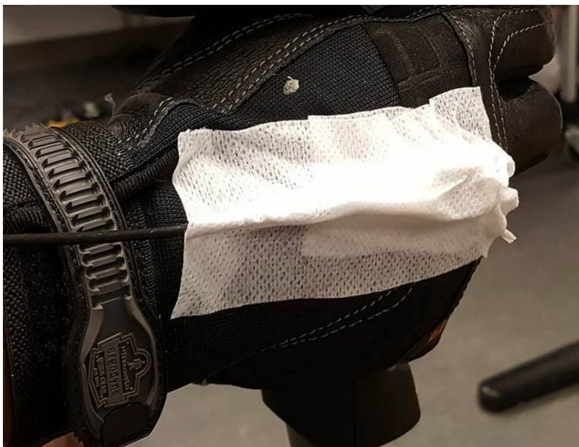
Figure 6: Position of accelerometer on the back of the hand.
