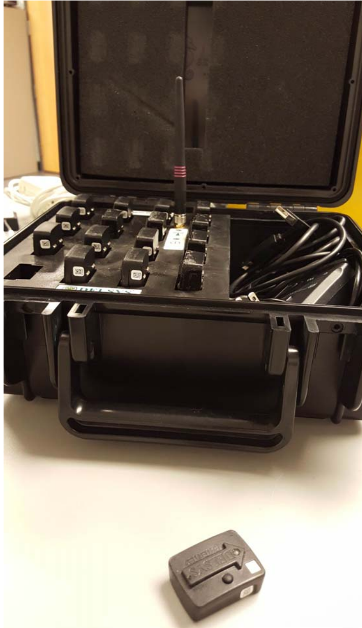
Figure 9: Trigno Delsys wireless EMG system.
