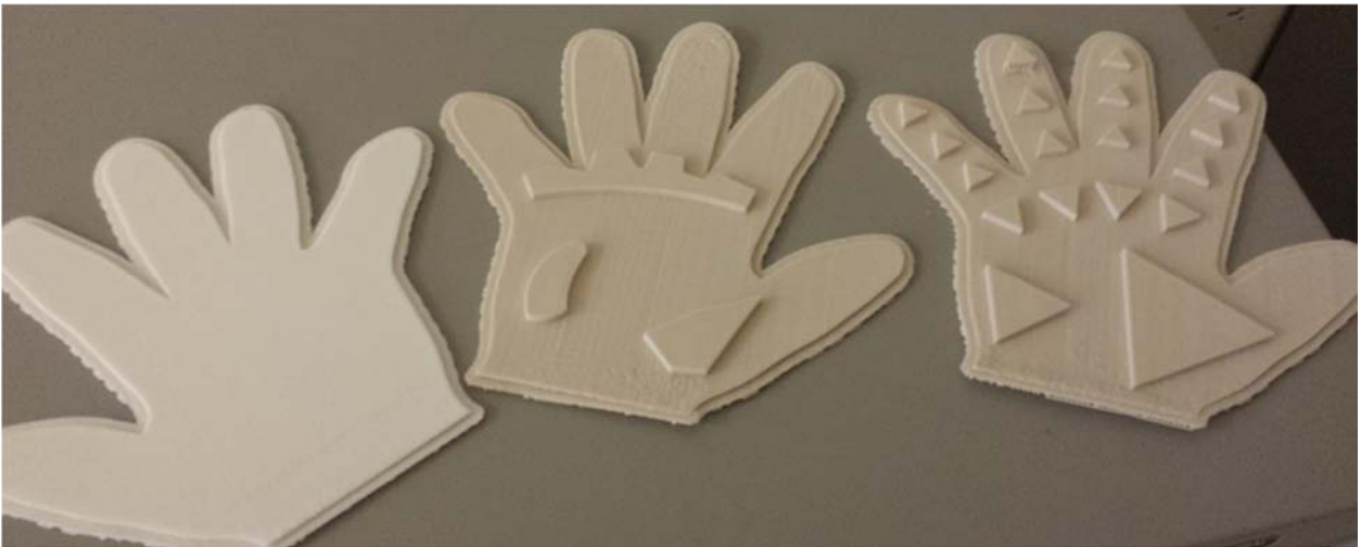
Figure 1: Left/Middle, two examples of AutoCAD designs and Right, a 3-D hand perspective of another design. Each design included a base layer (difficult to see in the perspective shown) and additional thick layers strategically placed.
