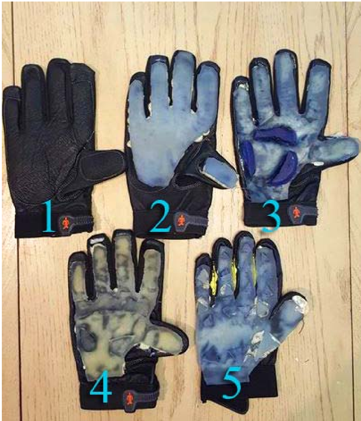
Figure 3: AV gloves tested. Glove 1: Standard Ergodyne 5mm Foam Glove (Proflex 9002 by Ergodyne Saint Paul, Minnesota, USA); Glove 2: 7mm gel-insert; Glove 3: 4mm gel-insert with 7mm palm inserts; Glove 4: 5mm gel-insert with 4mm palm inserts; Glove 5: 4mm gel-insert with 4mm triangular finger-to-palm inserts. Note: Gloves 2, 3 and 5 had the same gel composition as the base layer (but thickness varied). The thicker inserts on Glove 3 had a gel with different material properties than the base layer. Glove 4 consisted of a gel base and thicker insert pieces that had different material properties from Gloves 2, 3 and 5.
