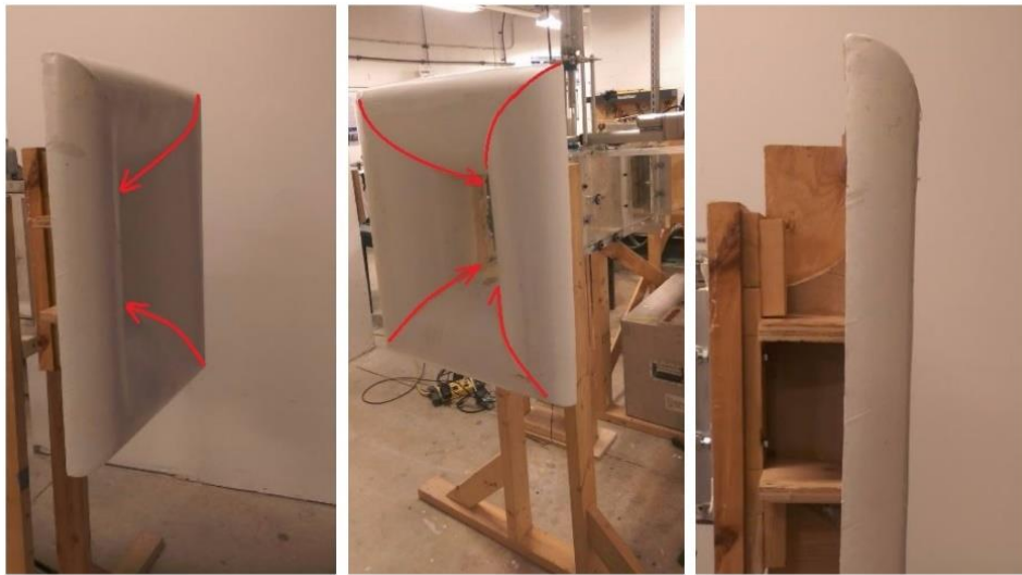
Figure 3-4 : Bellmouth for one of the used test sections
