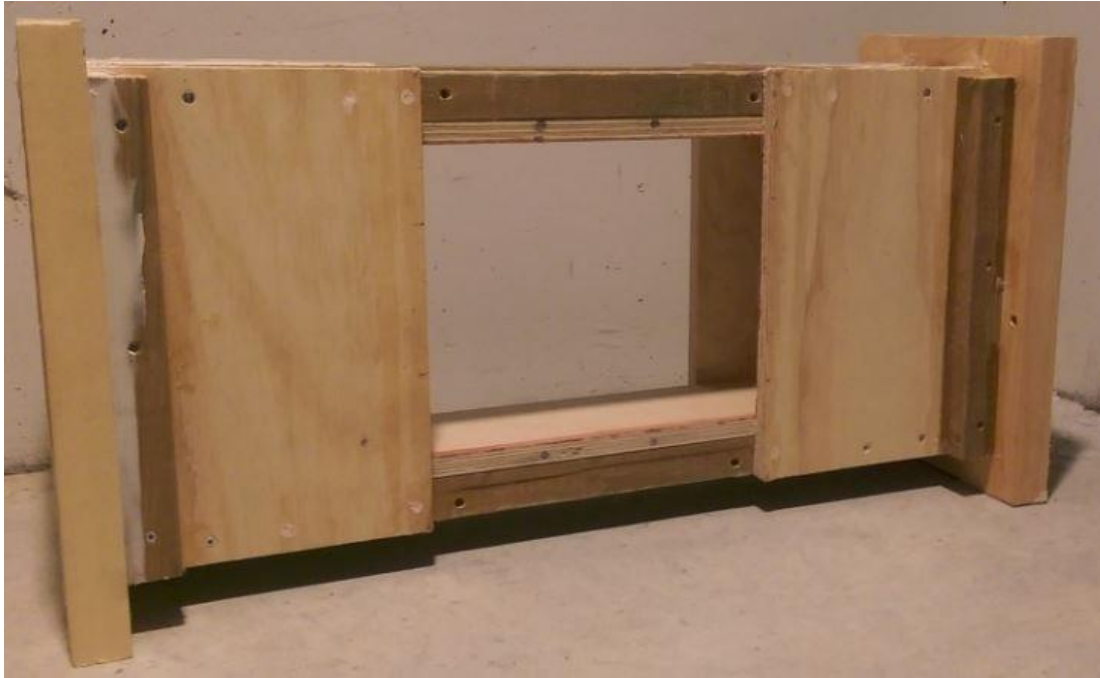
Figure 3-2 : Test section without the middle side windows
