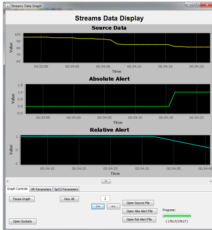
Figure 45. Streams Data Display application showing raw SpO 2 , SpO 2 absolute alert, SpO 2 relative alert
