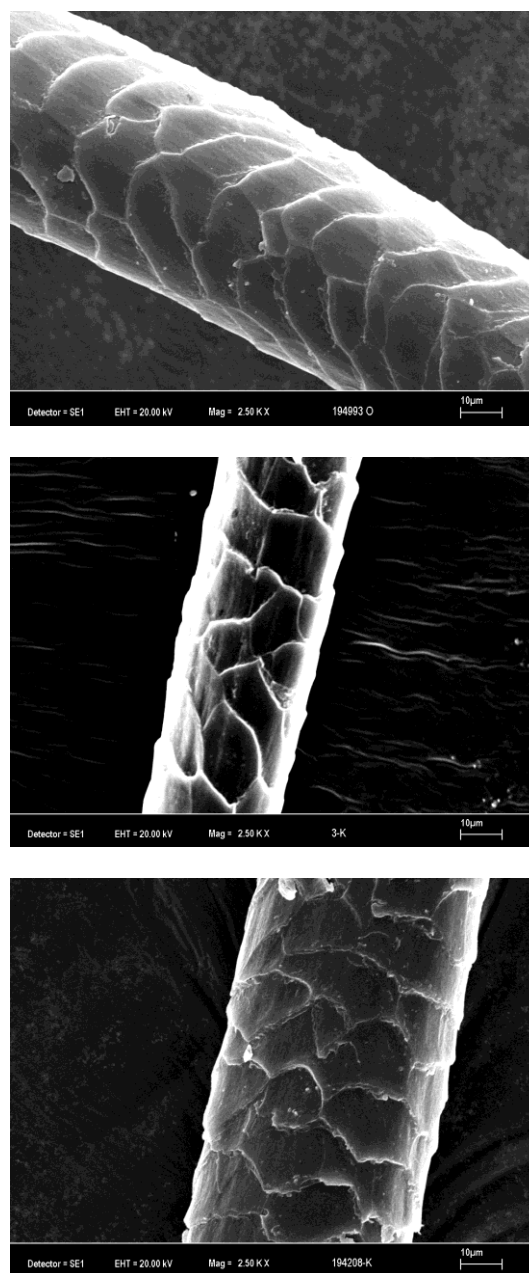
Figure 1. SEM Image of the fleece fiber in Menemen Sheep
