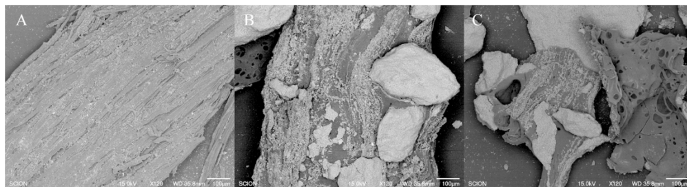
Figure 2. SEM images of char products mixed with used catalyst collected from catalytic fast pyrolysis experiments, AL360L (A), AL450L (B) and AL500L (C).
