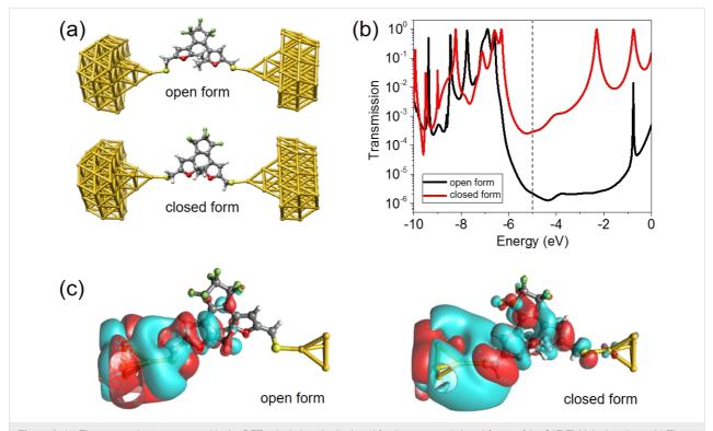
Figure 2: (a) The geometric structure used in the DFT calculations is displayed for the open and closed forms of Au-C5F-ThM-Au junctions. (b) The computed transmission curves for the open (black) and the closed form (red). (c) The wavefunction of the dominant transmission eigenchannel for electrons coming in from the left side for the open (left) and the closed form (right). Red and turquois indicate different signs of the wavefunction.
