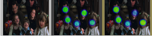
Figure 3. (Left) Input image. (Middle) The smile intensity heat map computed via MAEM. (Right) The smile intensity heat map computed via MAEM w . It is evident that larger faces get a higher weightage.
