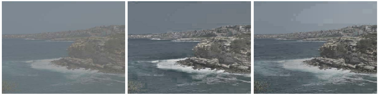
(b) (Left): Original image (Centre): Output of the proposed algorithm in the L*a*b* space (Right): CLAHE output in the L*a*b* space.
