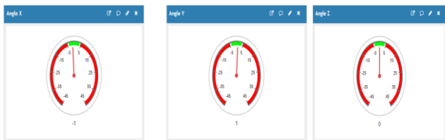
Fig. 10 Tilt angles for X, Y, Z before the pantograph passed the NS
