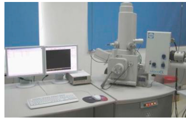
Fig.7 SEM used for wear morphology
