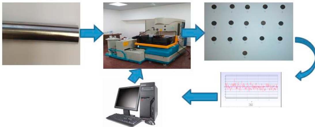
Fig. 1. Experimental setup for WEDM of Ni 55.8 Ti.
