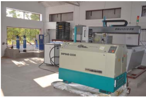
Fig. 1 Abrasive water jet cutting machine used in the present work. Fig. 2 Micrograph of hard abrasive particle used for AWJC
