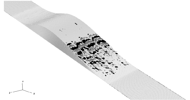
Fig. 15. The DMD mode for S_t = 2 computed from the flow around the bump, illustrated using two opposite contours of the perpendicular velocity component \mathbf{u}_{\perp} .
