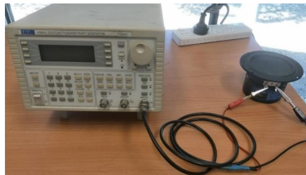
Figure 3.3. A 4-inch woofer speaker is attaching to a TTI 40 MHz DDS function/arbitrary generator.
