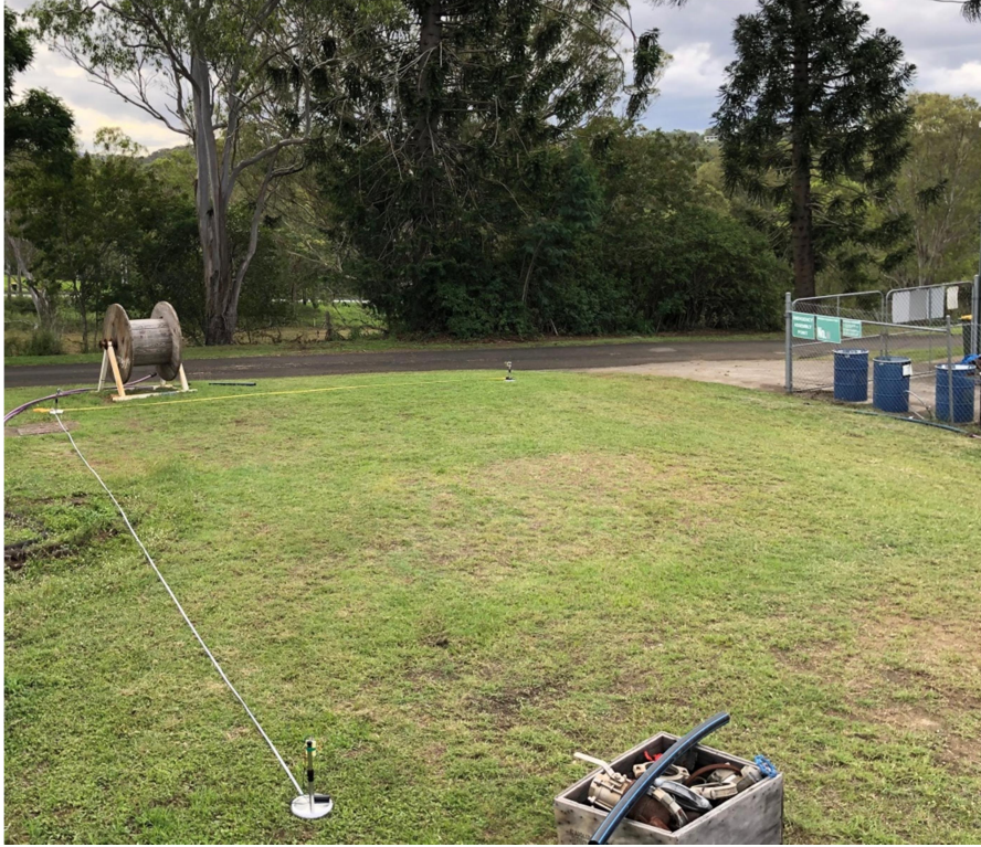
Figure 15: Outdoor Test Environment for UWB Beacons
