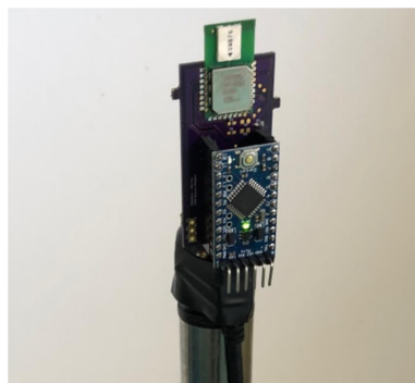
Figure 8: UWB Beacon with IC and Microcontroller
