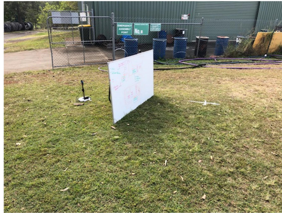
Figure 29: Whiteboard as test obstruction in front of the beacon
