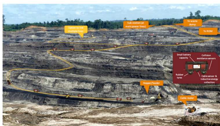
Figure 1: Proposed System Architecture of Autonomous Hauler [2]
