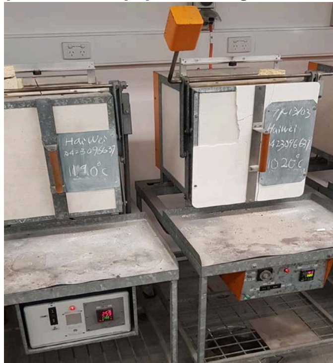
Figure 58: Furnace used for destabilization treatment & tempering
