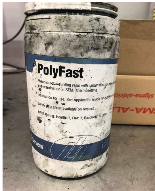
Figure 59: Polyfast resin used for sample mounting
