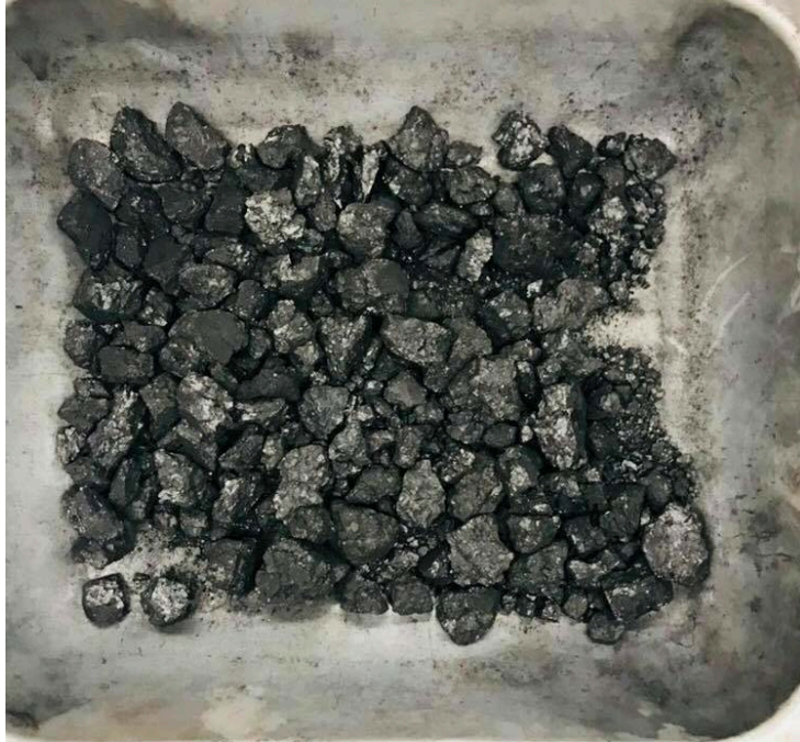
Figure 60: Coke used to prevent oxidation during heat treatment
