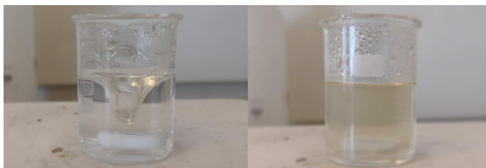
Figure 15 Viscosity Comparison of 0.2 wt% iCar Solution (left) and 2.7% iCar Solution (right)
