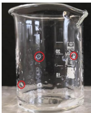
Figure 21 Solution #5 (iCar_0.2wt%_40°C) with agglomerates in red circle
