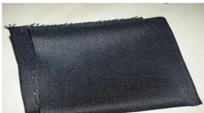
Figure 5. Carbon cloth electrode (Arungovind, Purushotham, Arunkumar, & Sendilvelan, 2017).
