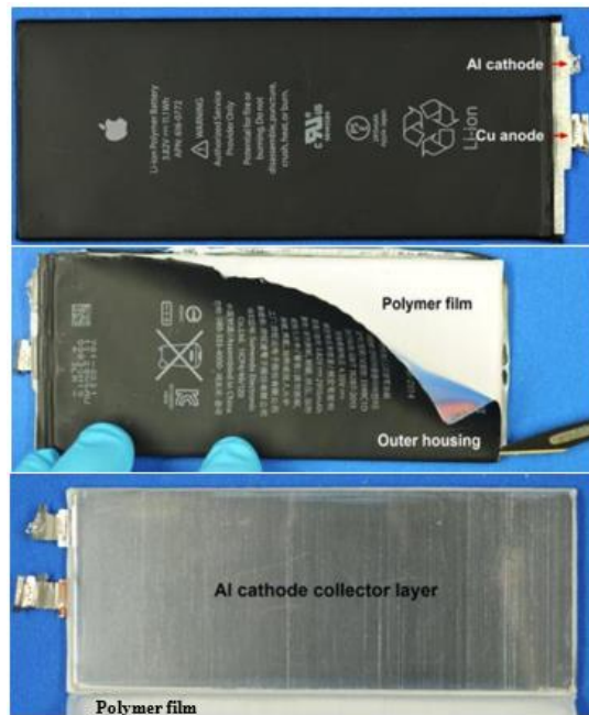
Figure 4.1 – Spent iPhone battery dismantling
