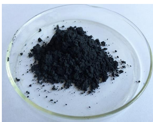
Figure 4.3 – LCO powder achieved from spent iPhone batteries
