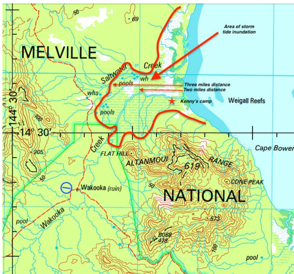
Figure 2.10 Topographical map of Wakooka Creek showing in red the area generally below 13 metres elevation (from NATMAP, Geoscience Australia).
