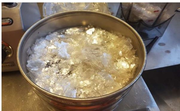
Figure 3-8 – Muscovite sheets after 2 minutes in the 800 W blender
