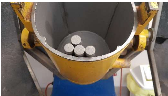
Figure 3-6 – Rod mill used for the grinding of pyrite and arsenopyrite
