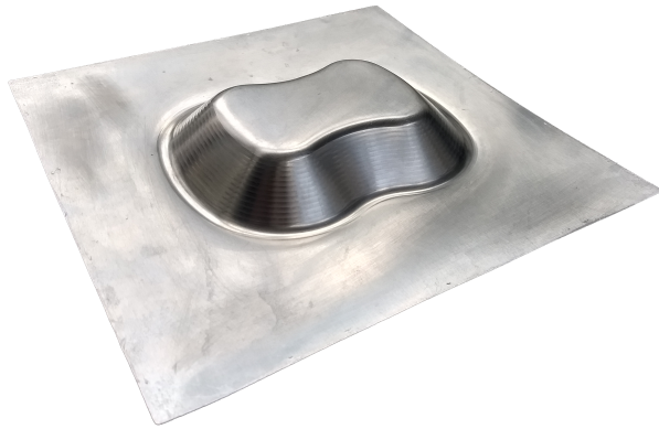
Figure 4.14: A photograph of the formed part (TPIF).
