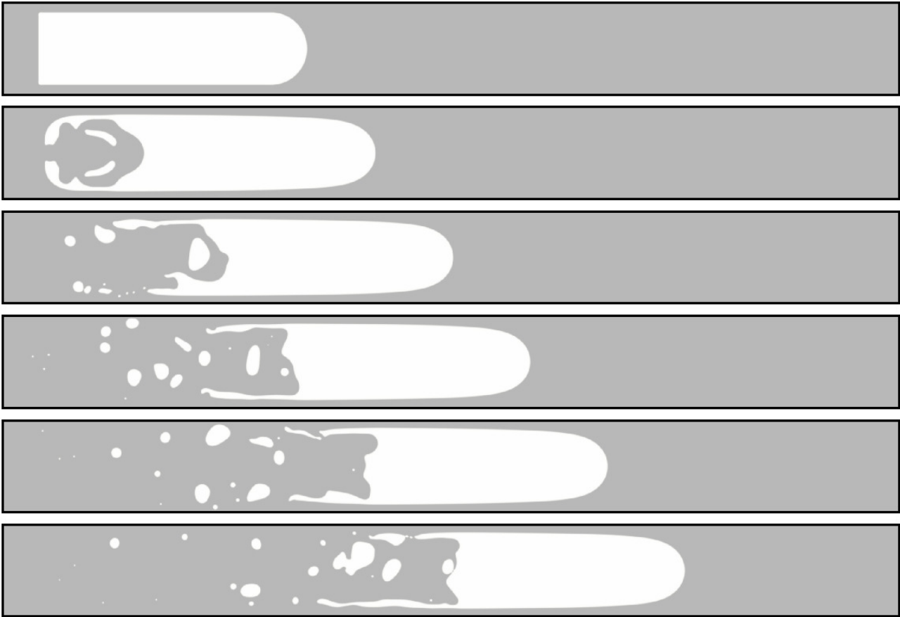
Figure 4.12: The time evolution of the planar Taylor bubble with snapshots taken at t^* = 0, 4, 8, 12, 16, 20 . The fluid properties are defined by \rho^* = 1000 and \mu^* = 100 , while the flow condition is specified through Re_r = 200 and Eo = 100 .
