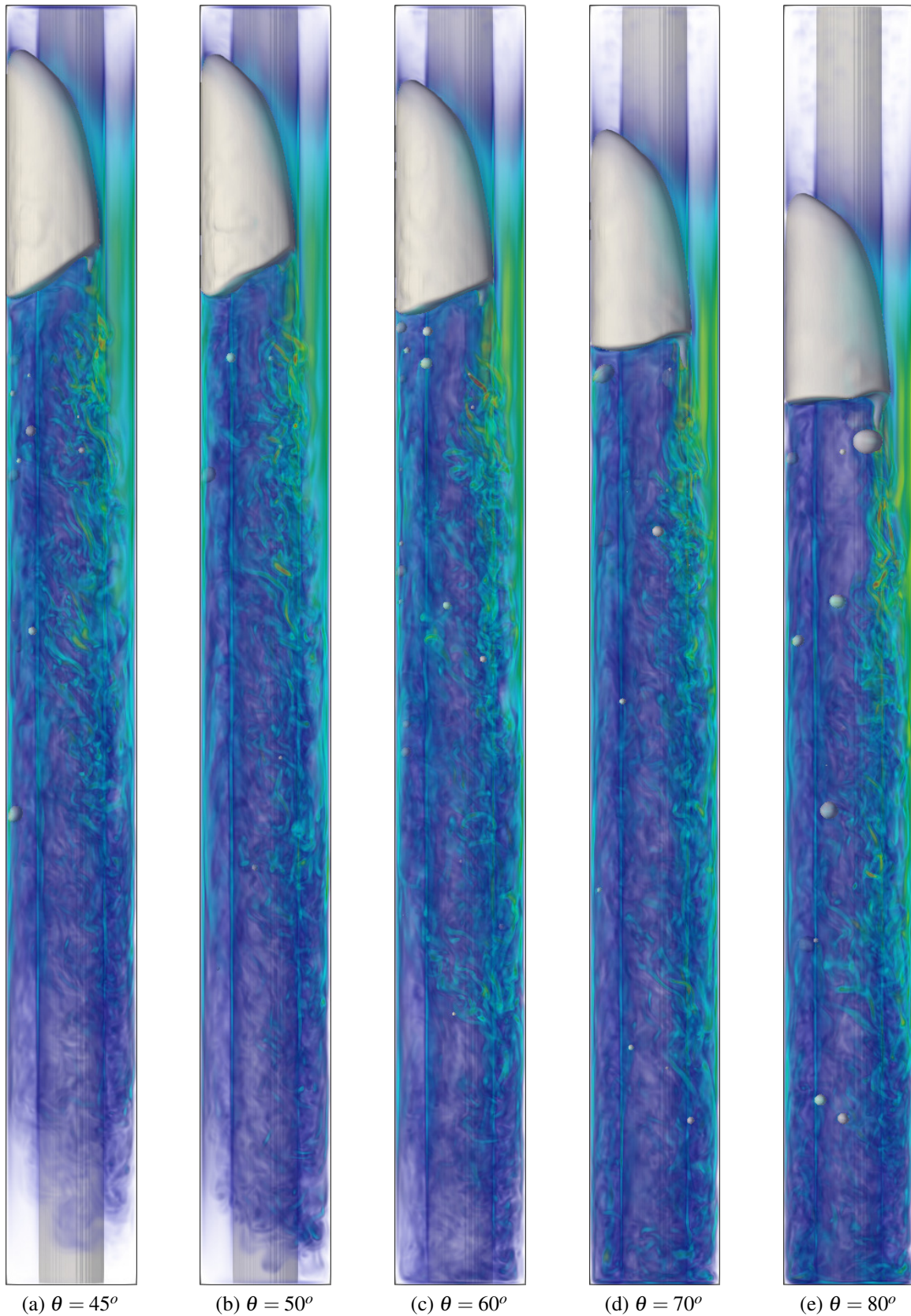
Figure 7.5: Taylor bubble profiles at t^* = 20t_0 with fluid parameters according to Case 3 ( Mo=2.56e-11 , Eo=21.65 ) and for pipe inclination angles (a) \theta = 45 , (b) \theta = 50 , (c) \theta = 60 , (d) \theta = 70 , (e) \theta = 80 degrees.
