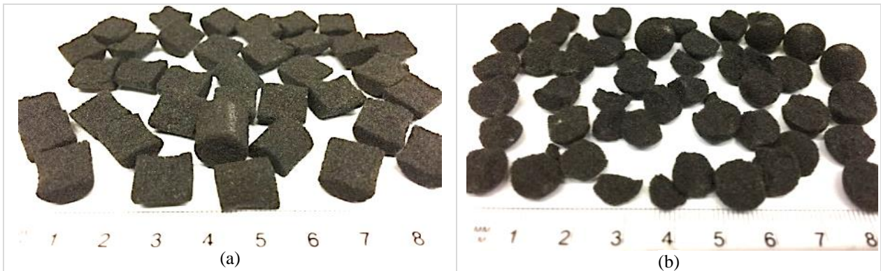
Figure 45 Pattern fracture for major fragments of 3DP with \approx 12.2 mm diameter: a) cylinder-shaped specimens printed horizontal and b) sphere-shaped specimens.
