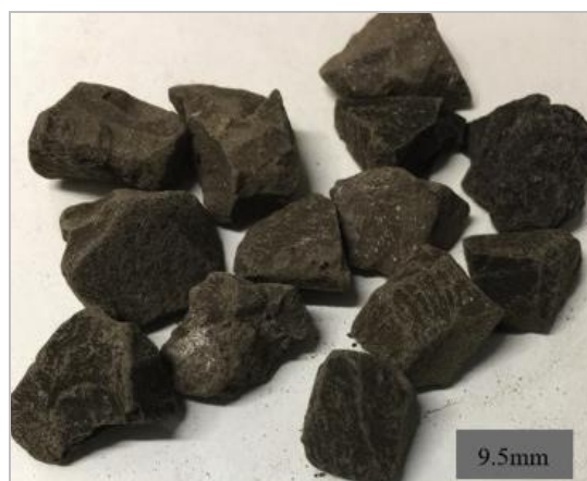
Figure 63 Illustration of irregular single-particles of mudstone tested on SILC.
