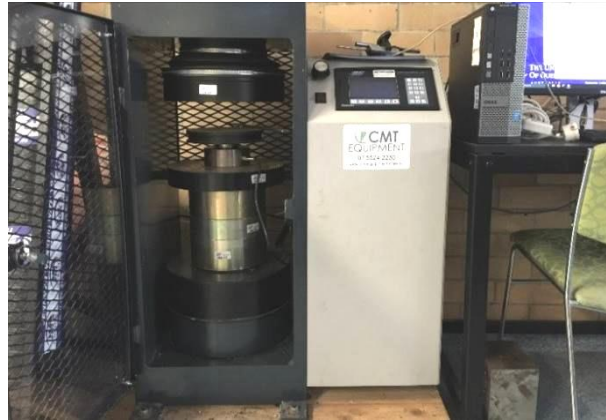
Figure 13 Photograph of the UCS testing machine used for mini-cylinder specimens.
