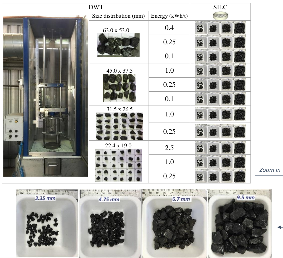
Figure 61 Illustration of the DWT used for fragmentation of distinct size distribution and varied energy in preparation for the irregular-particle specimens of coal tested on SILC.
