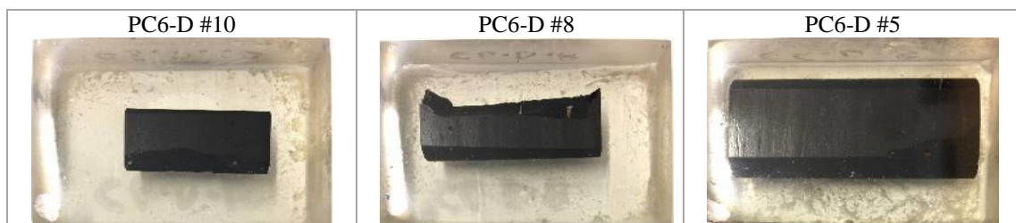
Figure 14 Examples of mini-cylinder specimens previously tested for UCS and prepared for petrographic analysis (blocks sized 50x30x12 mm).
