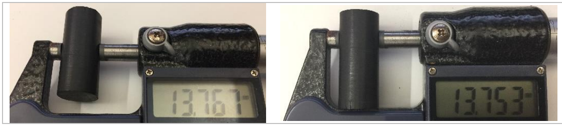
Figure 11 Example of one mini-cylinder being verified for the cylindrical profile of lateral walls.
