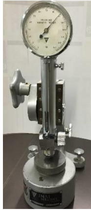
Figure 87 Shore scleroscope rebound hardness made by IMAI SIKENKI Co.
