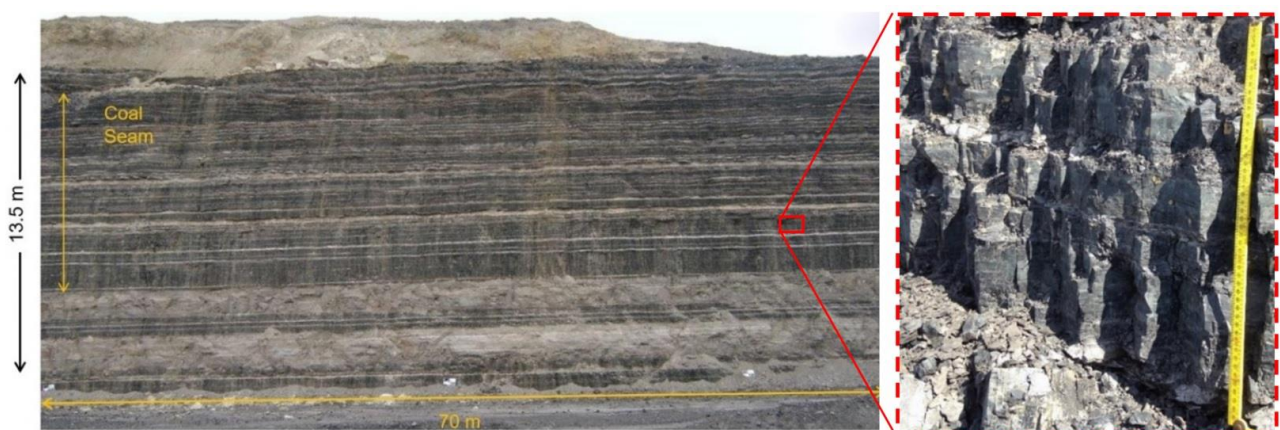
Figure 8 Illustration of Walloon Coal Measures showing variation in lithological units, and typical interbedded and banded nature of the plies (ruler stick is 50 cm long) (highwall photo courtesy of New Hope Mine).
