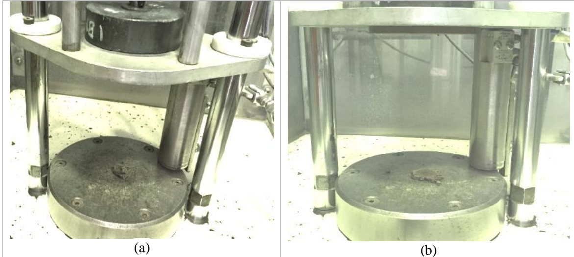
Figure 62 Evidence of ductile deformation for mudstone during fragmentation. a) before DWT test, b) after DWT test.
