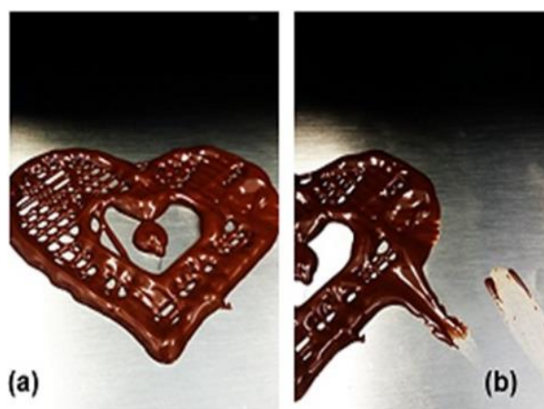
Figure 3.12: The effect of improper temperature setting on dark chocolate after extrusion (a) extruded chocolate at high temperature ( >36\text{ }^{\circ}\text{C} ) (b) chocolate was not solidified and collapsed during extrusion.
