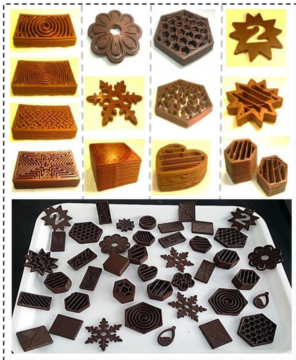
Figure 7.4: Various shapes, designs and internal structures (infill patterns and percentages) of 3D printed chocolates used in display session.
