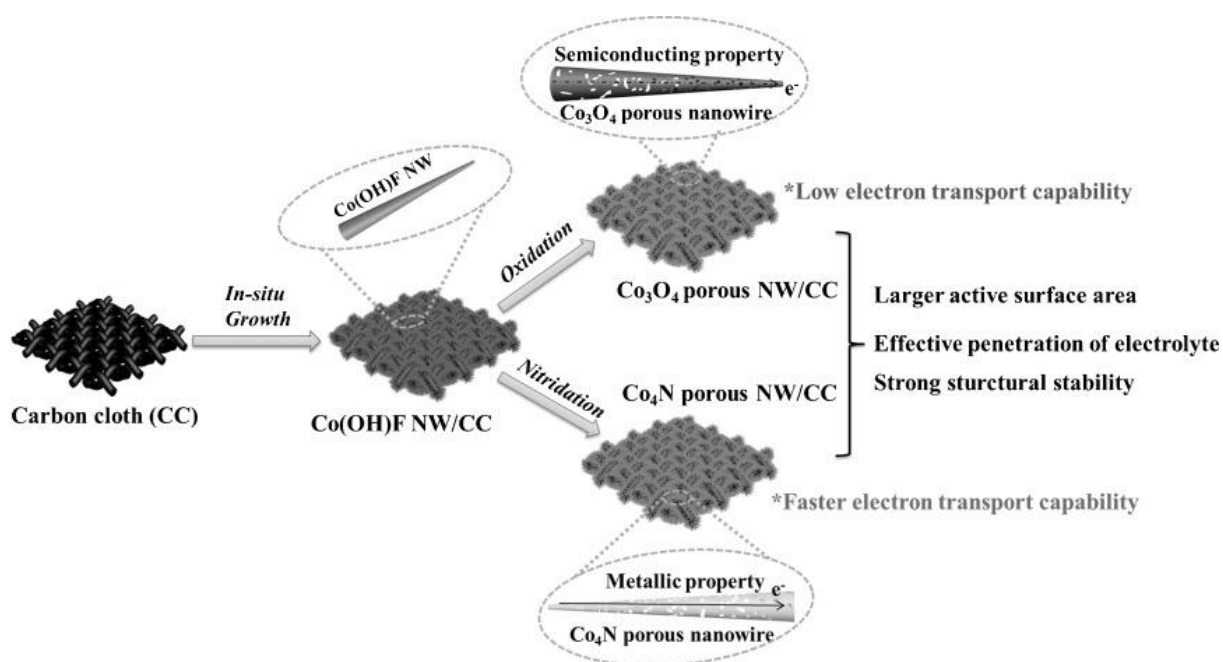
Figure 2-5. Schematic illustration of preparation for Co 4 N nanowire growing on carbon cloth. [32] Reproduced with permission from ref [32] . Copyright 2015, John Wiley and Sons.
