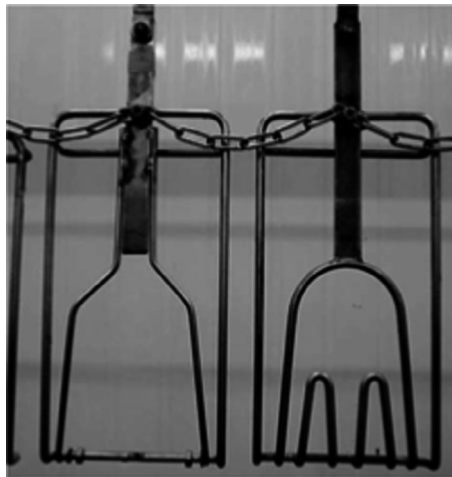
Figure 18: Compliant shackle (left) and standard plant shackle (right) installed in a processing plant. Reprinted by permission from: Universities Federation for Animal Welfare (UFAW), Lines et al., 2012
