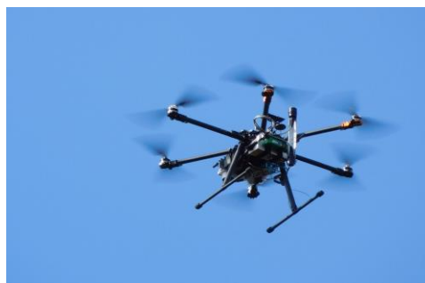
Figure 1. Hexacopter platform with Piccolo Doppio spectrometer system in flight. On this platform, the upwards and downwards pointing fore-optics are fixed in place using an aluminum strut, in the skywards and nadir directions respectively.
