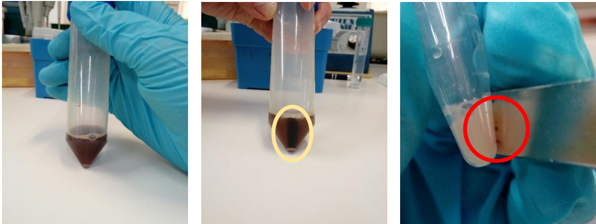
Figure 4.4: Preliminary magnetism tests. Left: Dex-70 coated IONP suspension. Centre: Dex-70 coated IONP suspension after brief exposure to a permanent magnet. Right: Magnetosome precipitate drawn to the magnet.
