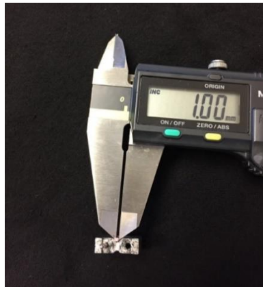
Figure 3.3.7 – Measurement of stick's bonding area with a digital micrometer.
