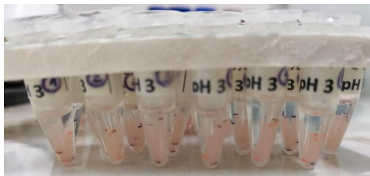
Figure 3.3.4 – specimens in graduated falcon tubes with artificial saliva.
