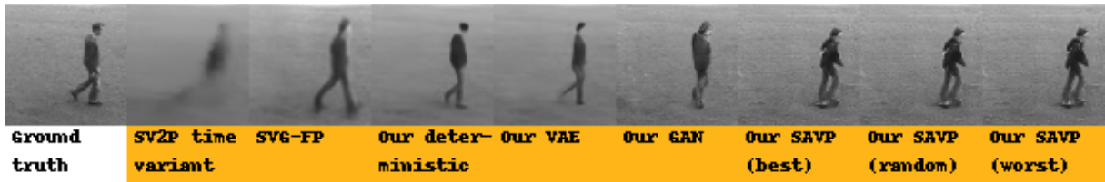
Figure 2.8: Prediction of future frames. On the extreme left the image represents the ground truth image from a clip of a man walking from left to right. On the right where the yellow tag is placed each box represents a prediction for what that ground truth image should be given an input of a history of past frames [3].
