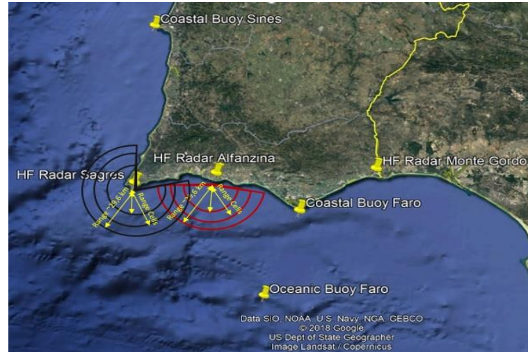
Figure 2.01: Algarve shore HF radar network and ODAS buoys systems used in this study. A descriptive HF radar range and range cell discretization are also represented for the Sagres and Alanzina radar sites.
