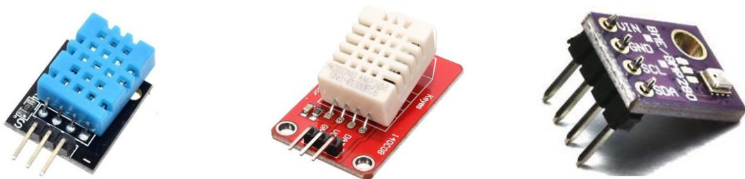
Figure 8 - T and RH Sensors; DHT11, DHT22 and BME280 in presentation order
