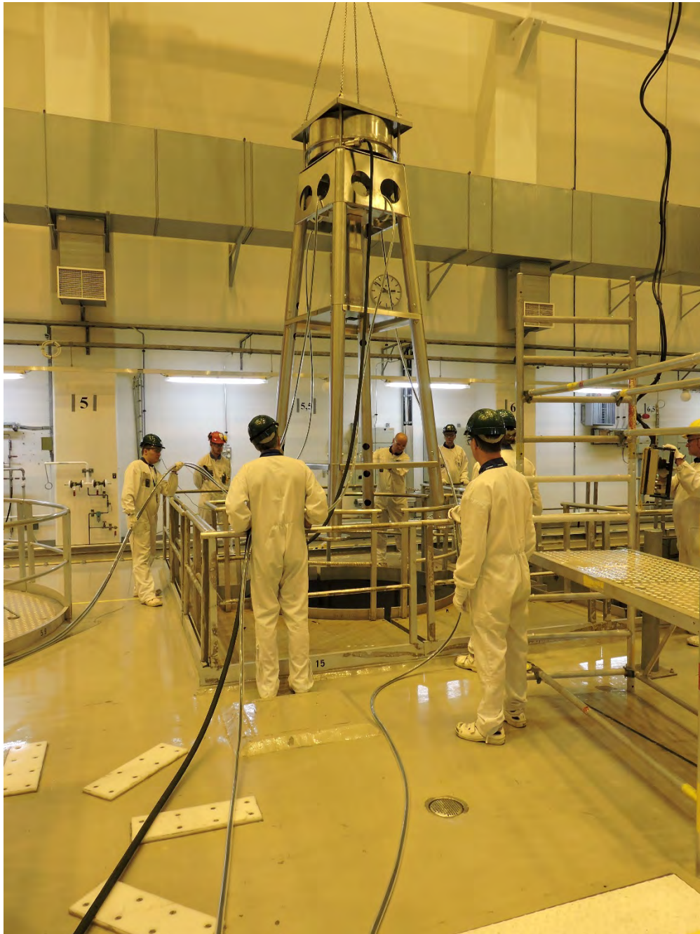
Figure 2. Setting up measurement campaign with PGET and PNAR in Olkiluoto Spent fuel Storage, July 2019.
