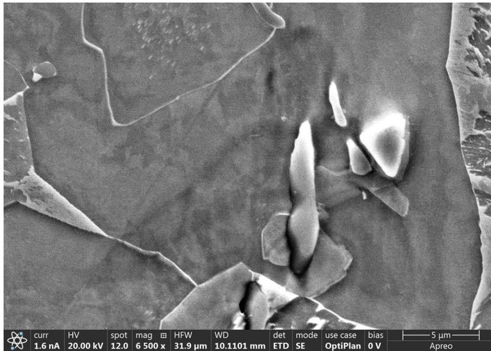
Figure 95: TiN and MnS precipitation in slow ACRT forging condition for steel M3
