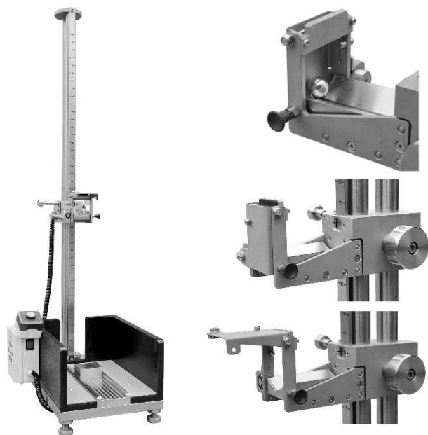
Figure 1. OZM BIT-132 (left side) and its release mechanism (right side).
