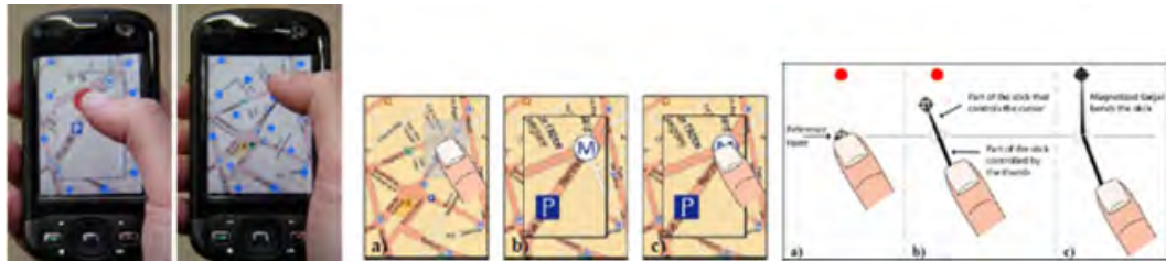
FIGURE 42 – From left to right : TapTap and MagStick interaction techniques, TapTap Design, MagStick Design
