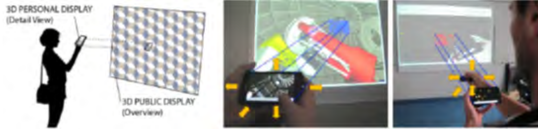
FIGURE 43 – the Mid-Air Phone technique and the Mid-Air Hand technique exploring 3D telescope visualization
