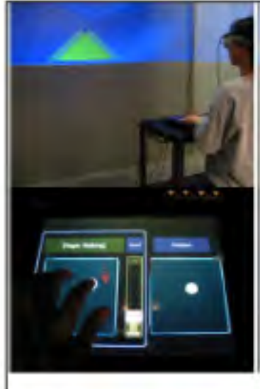
FIGURE 56 – Finger Walking in Place (FWIP) interaction technique
