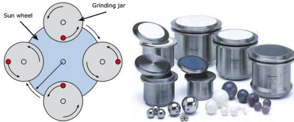
Figure 2.7: Speed ratios and grinding jar of Planetary Ball Mill
