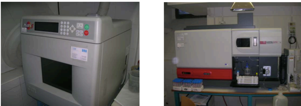
Figure 2: microwave oven CEM MARS-5 and ICP-AES Varian Vista MPX used for Hg determination.
