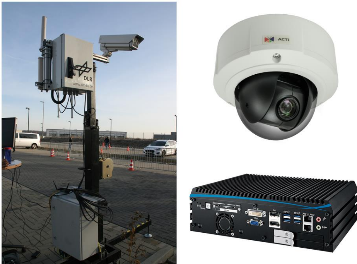
Figure 13: Mobile RSU with mounted ACTi Camera and ECX 1200 processing computer
