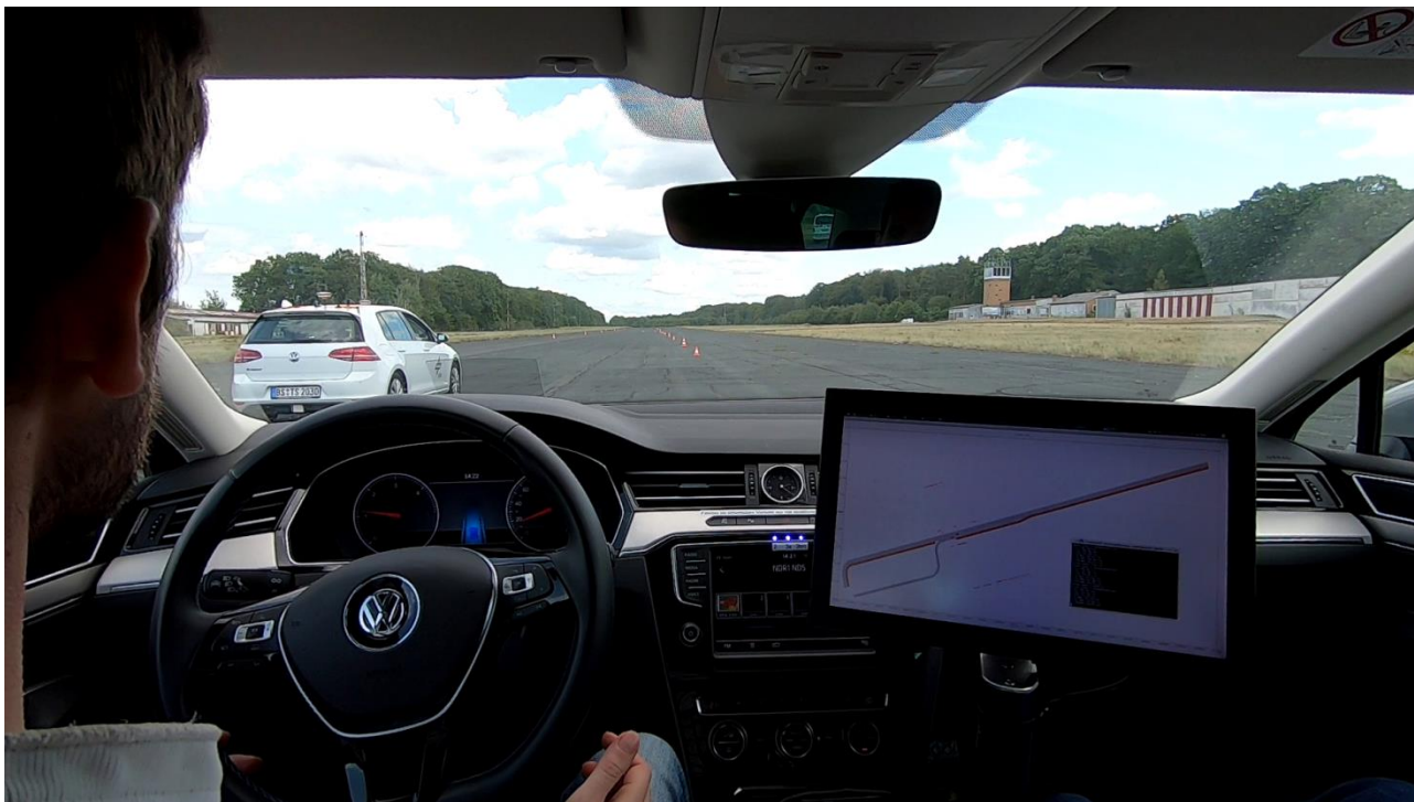
Figure 18: Blocked entrance, as manually driven FASCarE on adjacent lane does not allow merging (driving at the same speed). Lane change not possible, ViewCar2 stops.
