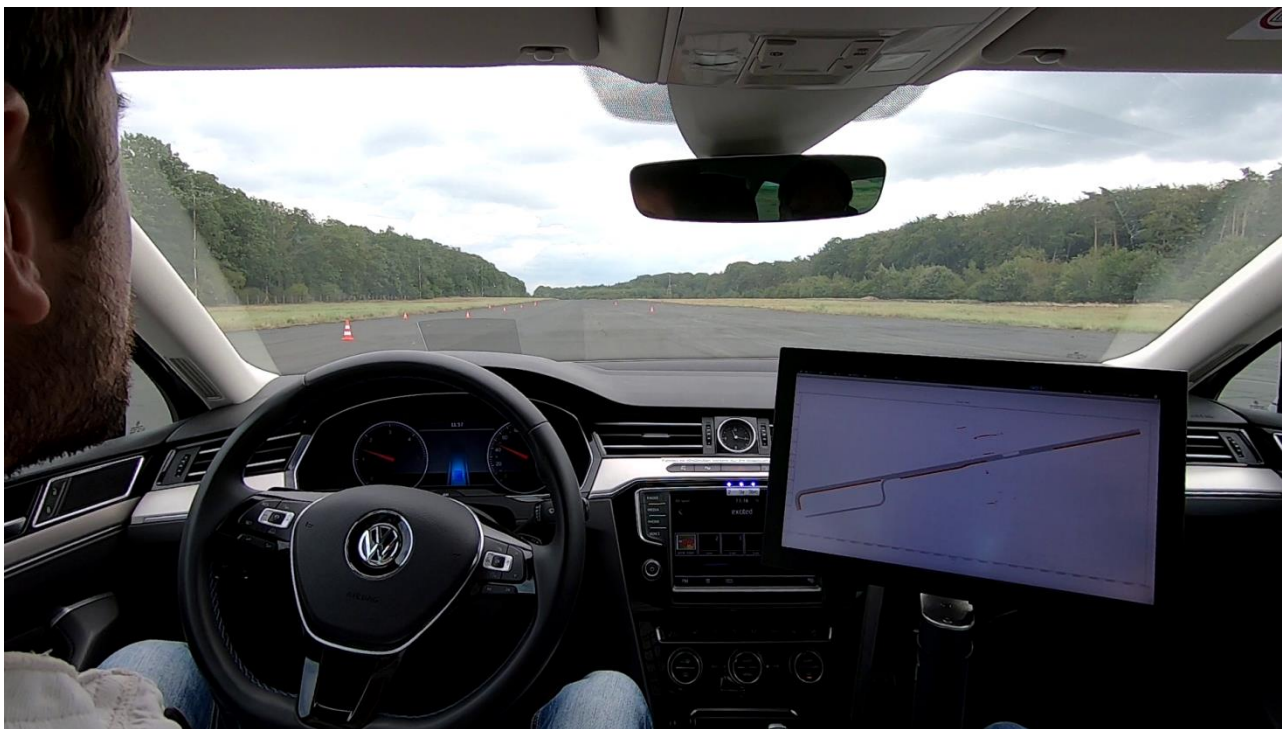
Figure 17: ViewCar2 executing the lane change around the blockage.
