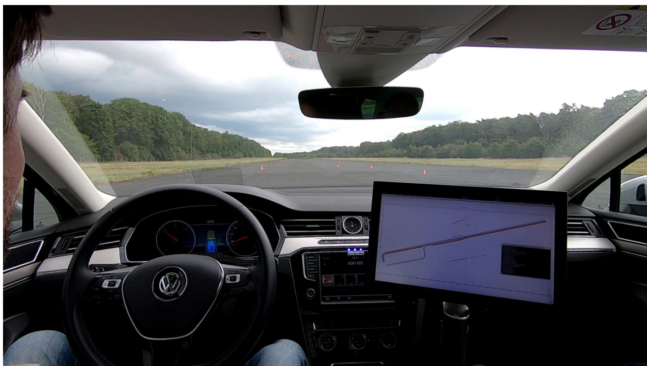
Figure 25: Internal view showing the received lane advice to the right lane in the cluster instrument
