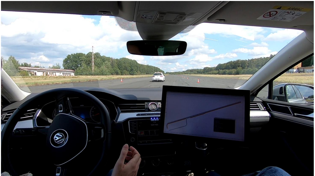
Figure 21: Successful lane change after speed adaptation of ViewCar2 on the ramp.
