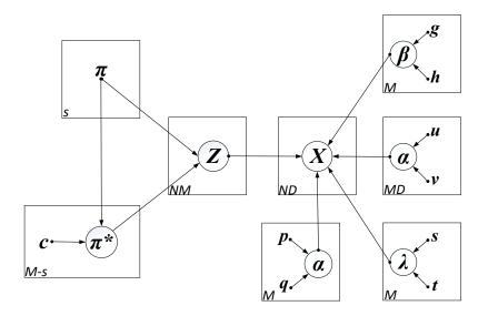
Figure 4.1: Graphical representation of IBL mixture model with component splitting. The circles indicate the random variables and model parameters, and plates point out the repetitions with the number in the lower left corners indicating the number of repetitions. The arcs specify the conditional dependencies of the variables.
